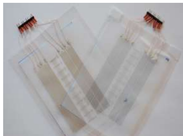
Fig. 4: Fabricated samples of capacitive level sensors with silver and semi-transparent PEDOT:PSS electrodes (IDC finger length 10mm)
