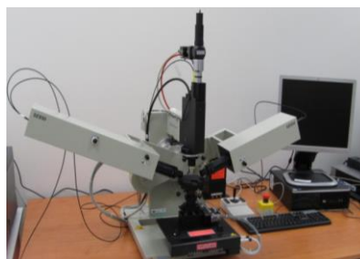
Obr. 25 – Elipsometr SENTECH SE850
