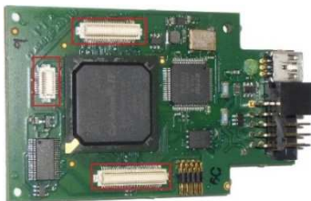
Figure 4-14 Interconnection – Side of the Base board
