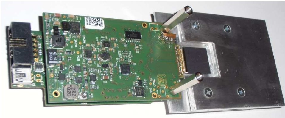
Figure 4-22 FITPix COMBO assembled with the additional aluminum cooler for the Timepix detector
