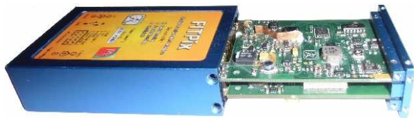
Figure 1-28 FITPix 3.0 Read-out interface (variant assembled with the serial interface board for Timepix)
