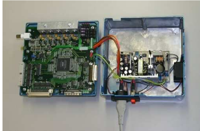
Figure 1-20 MUROS read-out interface (opened device casing)
