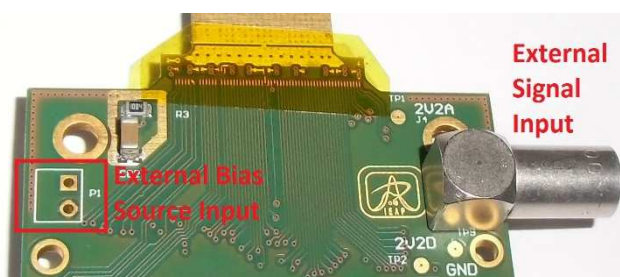
Figure 4-17 Detail of the PCB - External Signal input and external bias source input
