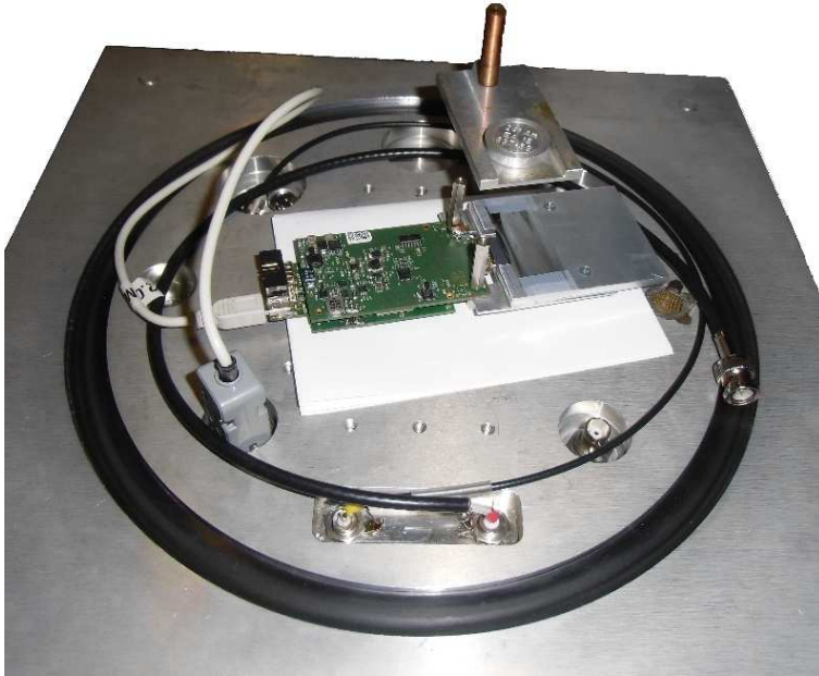
Figure 9-9 Arrangement of the FITpix COMBO device and Am alpha particle source in the vacuum chamber
