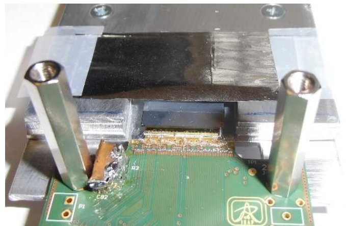
Figure 9-8 Detail view on the Timepix detector covered with the Mylar foil
