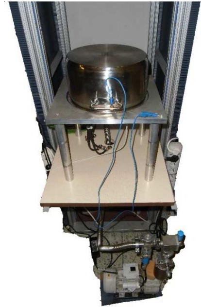
Figure 9-10 Vacuum chamber stand – experiment under progress
