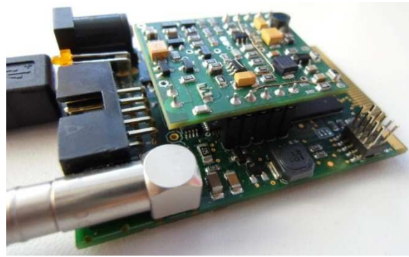
Figure 2-8 Detailed view on the uncovered Spectrig device (utilization of the FITPix hardware – bottom board. Additional spectro-module – top board)
