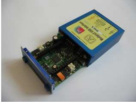
Figure 1-21 USB 1.1 Read-out interface (opened device casing)
