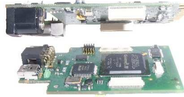
Figure 1-29 FITPix 3.0 (Detail of the sandwich assembly of the Base board and the Interface board)
