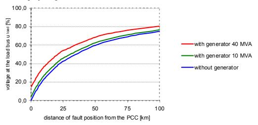
infeed is somewhat less. Before deciding about a double infeed it is necessary to find where most of the disturbing dips originate.
