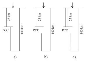
Figure 2 – Three alternatives of supply network: a) looped operation, b) radial operation and c) parallel operation
