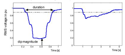
Figure 1 – Characteristics of a voltage dip caused by a) remote short-circuit fault and b) motor starting
