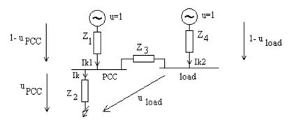
Figure 5 - Equivalent circuit for system with local generator
