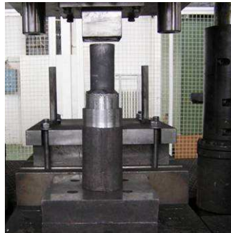
Figure 2. Compacting of packets on hydraulic press
