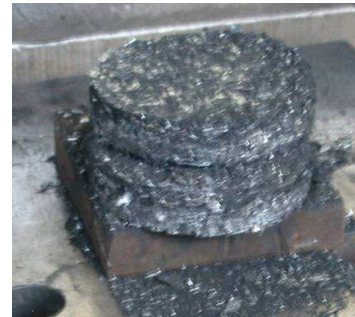
Figure 3. Packet of chips compacted with charcoal 1:6
