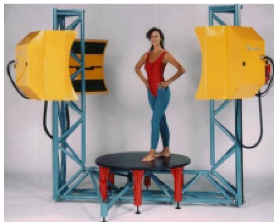
Figure 14. Cyberware 3D whole body scanner: Model WB4.
