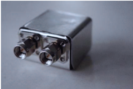
Fig. 4: Metal case for characteristics measurement
