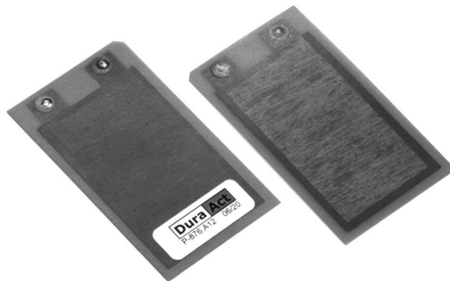
Fig. 2. Top and bottom view of the DuraAct P876.A12 piezoelectric transducers (patches)
