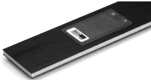
Fig. 1. Detail of sandwich beam with applied piezoelectric patch
