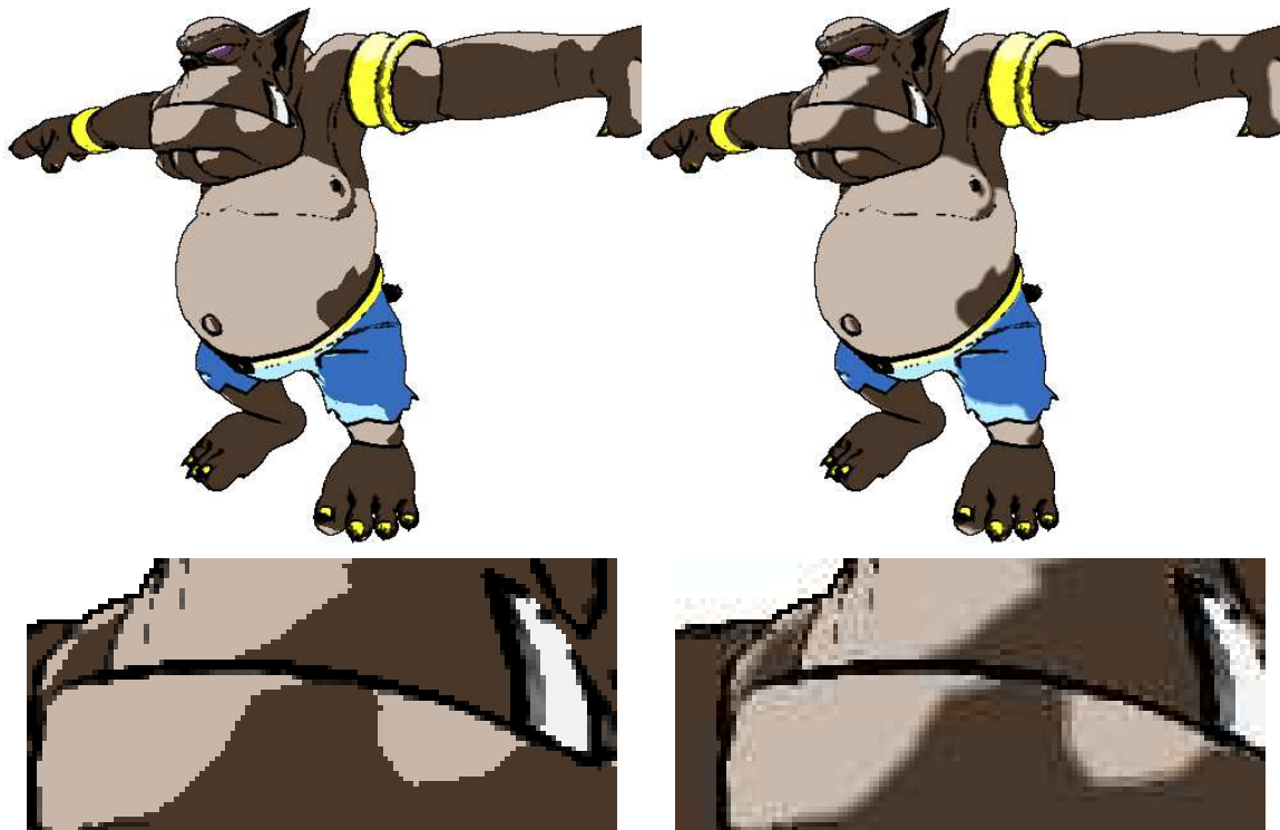
Figure 9: The edge-enhanced, cartoon-shaded “Olaf”. Nearest texture-filtering produces artifacts between consecutive color patches (left). Sampling neighboring color values smoothes color transition (right).
