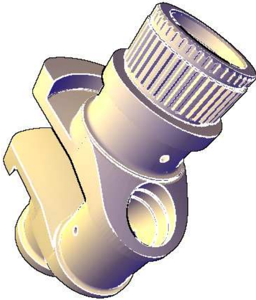
Figure 7: Gooch Illumination model for technical illustrations enhanced with different edge colors using the edge map. (Model used with permission)
