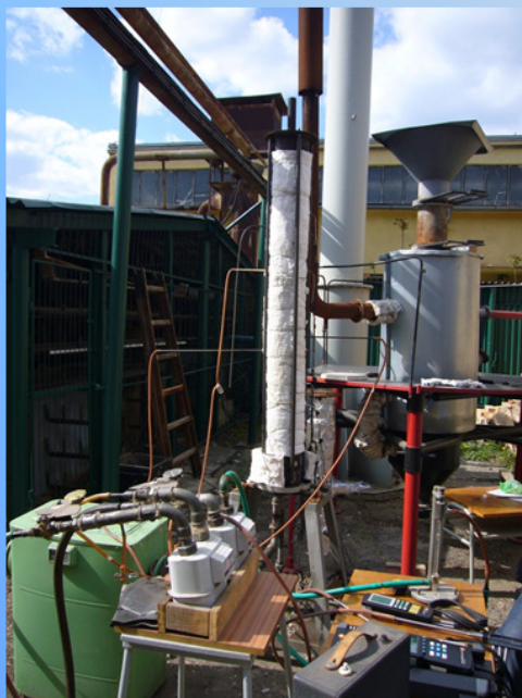
Fig. 5 Gasification device and reburning device
