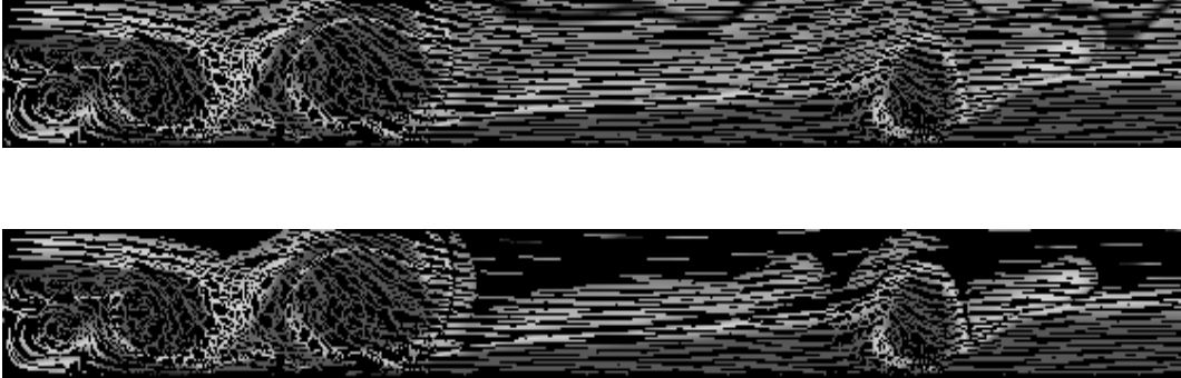
Figure 4: Vortex shedding past a backward facing step (laminar flow, Re=500 ).
