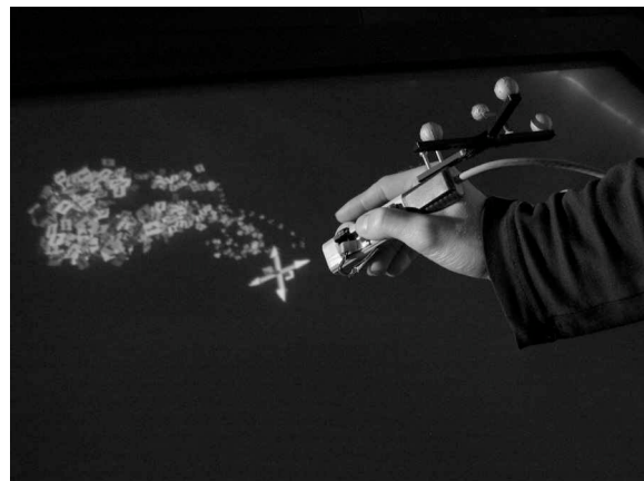
Figure 6: With the move tool objects not only can be moved but also scaled by using the scroll-wheel while the primary key is pressed.
