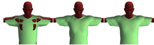
Figure 9: Left: coarse mesh, Centre: immediately after two adaption steps (incremental approach implies a change of one level for each step and level two is required in some areas to resolve the collisions), Right: after 1 second (30 adaption and 120 simulation steps), the cloth has relaxed.
