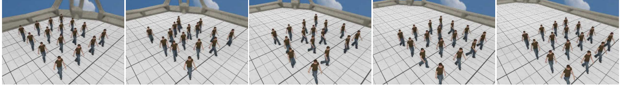
Figure 5: Self-organized reordering of a crowd with 16 characters. Control dynamics affects direction, distance and gait phase. See [Demo 7 ].
