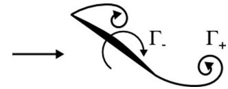
Fig. 2. Vortices formed on leading edge (leading edge vortex) and trailing edge (starting vortex)
