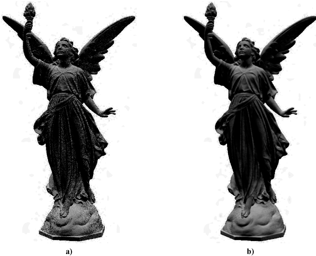
Figure 7. An image-space rendering of the Lucy model with artificial noise (a) without and (b) with luminance correction. The model was artificially up-sampled to 40 million points to achieve a high-enough point density. The normalization was again carried out over the weighted neighborhood. In this image the prevailing noise is less visible than in the torus rendering, since the surface shape of the model is not as homogeneous as the torus.
