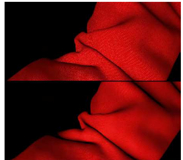
Figure 8: Level-of-detail rendering, without LOD (top) and with LOD (bottom).
