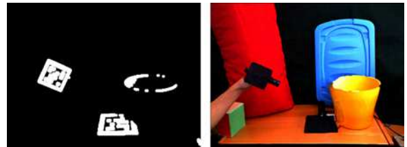
Figure 3: The left image shows the highlight mask. In a second step the masked pixels are filled as shown in the image on the right.
