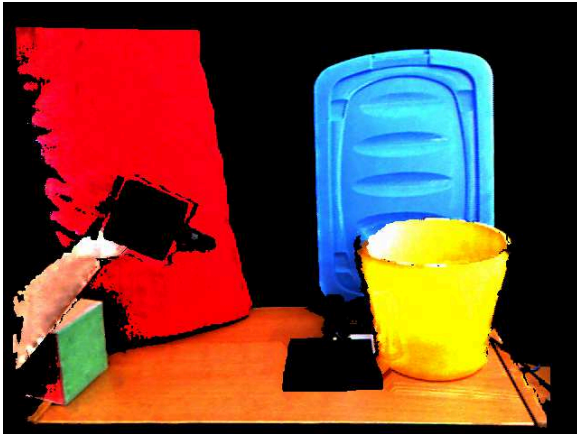
Figure 4: This image shows the estimated diffuse material component k_d . In the ideal case the objects would look perfectly flat and no variations due to different normals and thus illumination would be visible.
