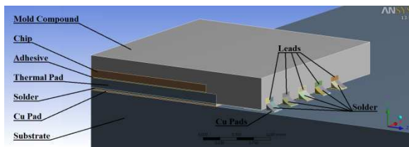
Fig. 2: Model of QFN package
